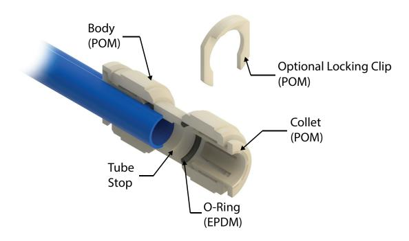
Push-to-Connect Fitting Cut-away Diagram
