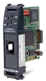
The H0-ECOM100 supports the Industry Standard Modbus TCP Client/Server Protocol
