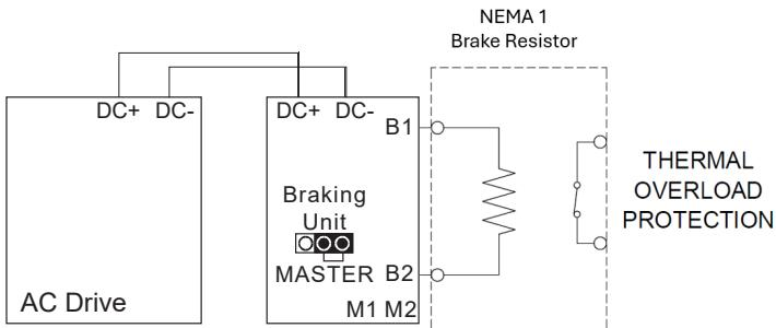
**Diagram F (Drive + DBUs with 1 Resistor or NEMA1 Resistor per DBU):**
