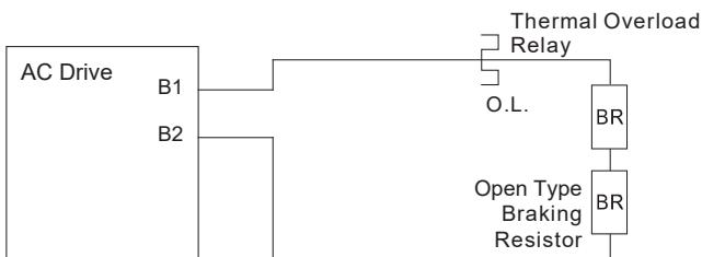
**Diagram C (Drive + 2 Parallel Resistors):**
