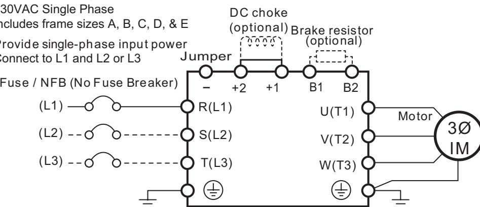
Connect 230VAC, Single-Phase power to any two of the R, S, or T terminals
