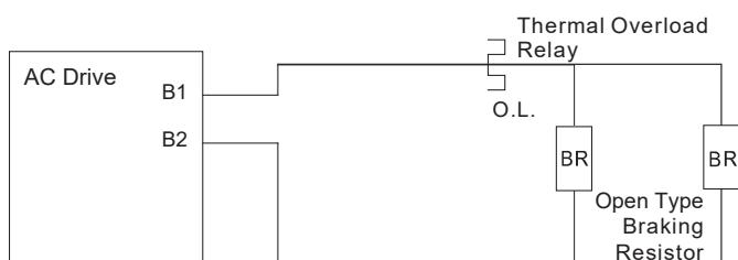
**Diagram D (drive + 2 Series and 2 Parallel Resistors):**
