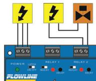
EchoSonic II (LU23, LU27, LU28 & LU29 Sensors & EchoPod (DL10, DL14, DL24 & DL34) Sourcing Mode (Factory Setting) Wiring Example:
