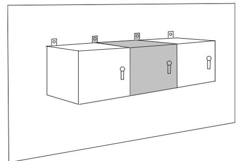
$$\text{Area (A)} = 1.4\text{ft}^2 [0.04\text{m}^2] (H \times W) + (H \times D) + 1.8\text{ft}^2 [0.05\text{m}^2] (W \times D)$$
