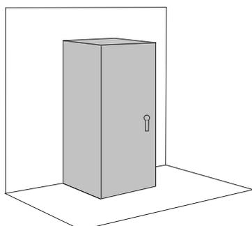
$$\text{Area (A)} = 1.4\text{ft}^2 [0.04\text{m}^2] (H \times W) + 1.8 (H \times D) + 1.4\text{ft}^2 [0.04\text{m}^2] (W \times D)$$
