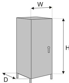
$$\text{Area (A)} = 1.8\text{ft}^2 [0.05\text{m}^2] (H \times W) + 1.8 (H \times D) + 1.8\text{ft}^2 [0.05\text{m}^2] (W \times D)$$
