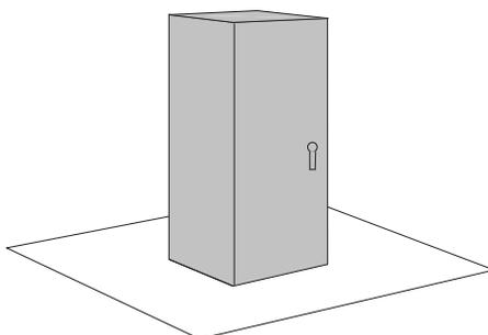
$$\text{Area (A)} = 1.8\text{ft}^2 [0.05\text{m}^2] (H \times W) + 1.8 (H \times D) + 1.4\text{ft}^2 [0.04\text{m}^2] (W \times D)$$
