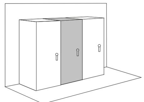
$$\text{Area (A)} = 1.4\text{ft}^2 [0.04\text{m}^2] (H \times W) + (H \times D) + 1.4\text{ft}^2 [0.04\text{m}^2] (W \times D)$$
