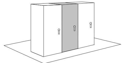
$$\text{Area (A)} = 1.8\text{ft}^2 [0.05\text{m}^2] (H \times W) + (H \times D) + 1.4\text{ft}^2 [0.04\text{m}^2] (W \times D)$$
