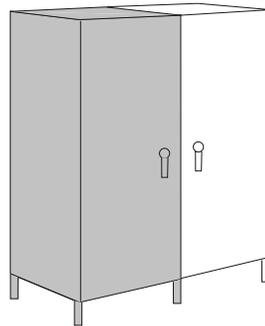
$$\text{Area (A)} = 1.8\text{ft}^2 [0.05\text{m}^2] (H \times W) + 1.4 (H \times D) + 1.8\text{ft}^2 [0.05\text{m}^2] (W \times D)$$
