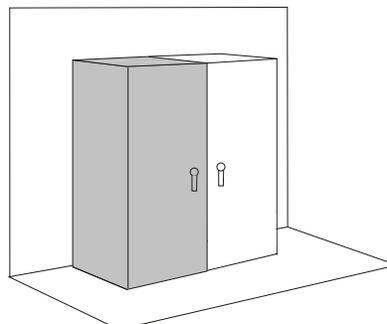
$$\text{Area (A)} = 1.4\text{ft}^2 [0.04\text{m}^2] (H \times W) + 1.4 (H \times D) + 1.4\text{ft}^2 [0.04\text{m}^2] (W \times D)$$
