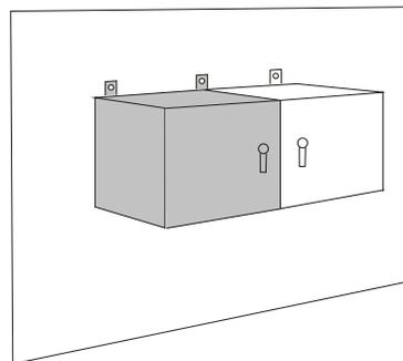
$$\text{Area (A)} = 1.4\text{ft}^2 [0.04\text{m}^2] (H \times W) + 1.4 (H \times D) + 1.8\text{ft}^2 [0.05\text{m}^2] (W \times D)$$
