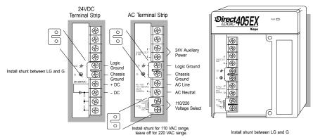
Recommended screw torque: 10.6 lb-in (1.2 Nm)
