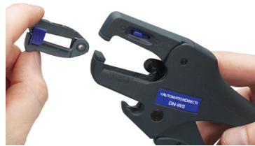
DN-WS stripping blade replacement
