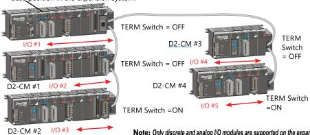
**Note:** Only discrete and analog I/O modules are supported on the expansion bases. No specialty or communications modules can be used on the expansion bases at this time.
