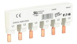
Eaton busbar, 80A, 480 VAC, cut to length not permitted, connects up to (2) 3-pole Eaton FAZ-NA series miniature circuit breakers without auxiliary components.
