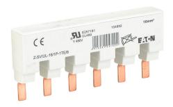
Eaton busbar, 80A, 480 VAC, cut to length not permitted, connects up to (6) 1-pole Eaton FAZ-NA series miniature circuit breakers without auxiliary components.
