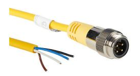
ZIPport connection cable, 7/8in - 16 UN2 thread nut 4-pin male axial to pigtail with European (Cenelec) color code, PVC outer jacket, yellow, nickel-plated brass connector, 19.6ft/6m cable length, IP67.
