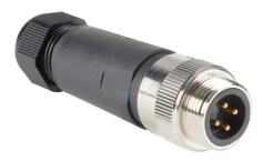
ZIPport field wireable connector, 7/8in - 16 UN2 thread barrel 4-pin male axial, accepts cable diameter size 5-13mm, 20 -14 AWG, screw terminal connection, European (Cenelec) color code, IP67.
