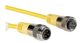
ZIPport connection cable, 7/8in - 16 UN2 thread barrel 4-pin male axial to 7/8in - 16 UN2 thread nut 4-pin female axial, PVC outer jacket, yellow, nickel-plated brass connector, 13.1ft/4m cable length, IP67.
