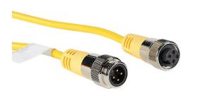
ZIPport connection cable, 7/8in - 16 UN2 thread barrel 4-pin male axial to 7/8in - 16 UN2 thread nut 4-pin female axial, PVC outer jacket, yellow, nickel-plated brass connector, 6.5ft/2m cable length, IP67.
