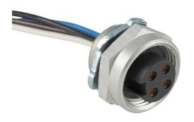
ZIPport bulkhead connector, 7/8in 4-pin female to pigtail, 18 AWG, 0.9ft/0.3m cable length, ether-based polyurethane conductor insulation material, IP67.
