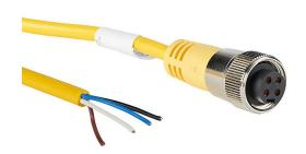
ZIPport connection cable, 7/8in - 16 UN2 thread nut 4-pin female axial to pigtail with European (Cenelec) color code, PVC outer jacket, yellow, nickel-plated brass connector, 13.1ft/4m cable length, IP67.
