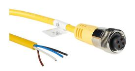
ZIPport connection cable, 7/8in - 16 UN2 thread nut 4-pin female axial to pigtail with European (Cenelec) color code, PVC outer jacket, yellow, nickel-plated brass connector, 6.5ft/2m cable length, IP67.
