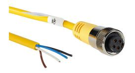
ZIPport connection cable, 7/8in - 16 UN2 thread nut 4-pin female axial to pigtail with European (Cenelec) color code, PVC outer jacket, yellow, nickel-plated brass connector, 32.8ft/10m cable length, IP67.
