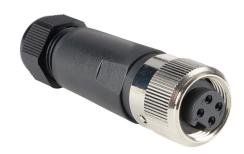
ZIPport field wireable connector, 7/8in - 16 UN2 thread nut 4-pin female axial, accepts cable diameter size 5-13mm, 20 - 14 AWG, screw terminal connection, European (Cenelec) color code, IP67.
