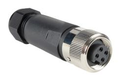
ZIPport connector, field-wireable, 7/8in - 16 UN2 thread nut 4-pin female axial, accepts cable diameter size 5-13mm, 20 - 14 AWG, European (Cenelec) color code, screw terminal connection, IP67.
