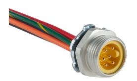
ZIPport bulkhead connector, 7/8in 6-pin male to pigtail, 16 AWG, 0.9ft/0.3m cable length, ether-based polyurethane conductor insulation material, IP67.
