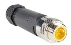
ZIPport field wireable connector, 7/8in - 16 UN2 thread barrel 6-pin male axial, accepts cable diameter size 5-13mm, 20 - 16 AWG, screw terminal connection, North American color code, IP67.
