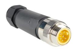
ZIPport connector, field-wireable, 7/8in - 16 UN2 thread barrel 6-pin male axial, accepts cable diameter size 5-13mm, 20 - 16 AWG, North American color code, screw terminal connection, IP67.
