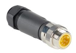
ZIPport connector, field-wireable, 7/8in - 16 UN2 thread barrel 6-pin male axial, accepts cable diameter size 8-17mm, 20 - 16 AWG, North American color code, screw terminal connection, IP67.
