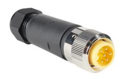
ZIPport connector, field-wireable, 7/8in - 16 UN2 thread nut 6-pin male axial, accepts cable diameter size 5-13mm, 20 - 16 AWG, North American color code, screw terminal connection, IP67.
