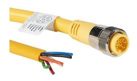
ZIPport connection cable, 7/8in - 16 UN2 thread nut 6-pin male axial to pigtail with North American color code, PVC outer jacket, yellow, nickel-plated brass connector, 13.1ft/4m cable length, IP67.
