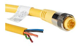
ZIPport connection cable, 7/8in - 16 UN2 thread nut 6-pin male axial to pigtail with North American color code, PVC outer jacket, yellow, nickel-plated brass connector, 32.8ft/10m cable length, IP67.
