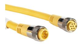
ZIPport connection cable, 7/8in - 16 UN2 thread nut 6-pin male axial to 7/8in - 16 UN2 thread nut 6-pin female axial, PVC outer jacket, yellow, nickel-plated brass connector, 19.6ft/6m cable length, IP67.
