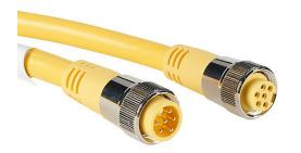
ZIPport connection cable, 7/8in - 16 UN2 thread nut 6-pin male axial to 7/8in - 16 UN2 thread nut 6-pin female axial, PVC outer jacket, yellow, nickel-plated brass connector, 13.1ft/4m cable length, IP67.
