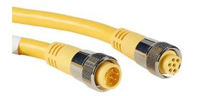
ZIPport connection cable, 7/8in - 16 UN2 thread nut 6-pin male axial to 7/8in - 16 UN2 thread nut 6-pin female axial, PVC outer jacket, yellow, nickel-plated brass connector, 6.5ft/2m cable length, IP67.
