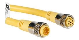
ZIPport connection cable, 7/8in - 16 UN2 thread nut 6-pin male axial to 7/8in - 16 UN2 thread nut 6-pin female axial, PVC outer jacket, yellow, nickel-plated brass connector, 32.8ft/10m cable length, IP67.
