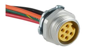
ZIPport bulkhead connector, 7/8in 6-pin female to pigtail, 16 AWG, 0.9ft/0.3m cable length, ether-based polyurethane conductor insulation material, IP67.
