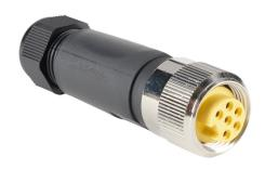
ZIPport connector, field-wireable, 7/8in - 16 UN2 thread nut 6-pin female axial, accepts cable diameter size 5-13mm, 20 - 16 AWG, North American color code, screw terminal connection, IP67.
