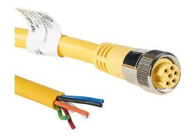
ZIPport connection cable, 7/8in - 16 UN2 thread nut 6-pin female axial to pigtail with North American color code, PVC outer jacket, yellow, nickel-plated brass connector, 19.6ft/6m cable length, IP67.
