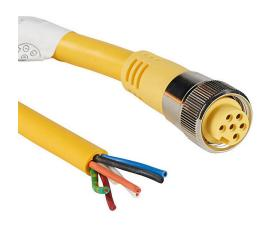
ZIPport connection cable, 7/8in - 16 UN2 thread nut 6-pin female axial to pigtail with North American color code, PVC outer jacket, yellow, nickel-plated brass connector, 13.1ft/4m cable length, IP67.
