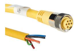
ZIPport connection cable, 7/8in - 16 UN2 thread nut 6-pin female axial to pigtail with North American color code, PVC outer jacket, yellow, nickel-plated brass connector, 6.5ft/2m cable length, IP67.
