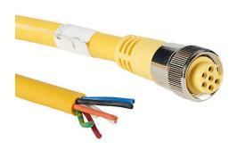
ZIPport connection cable, 7/8in - 16 UN2 thread nut 6-pin female axial to pigtail with North American color code, PVC outer jacket, yellow, nickel-plated brass connector, 32.8ft/10m cable length, IP67.
