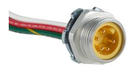
ZIPport bulkhead connector, 7/8in 5-pin male to pigtail, 16 AWG, 0.9ft/0.3m cable length, ether-based polyurethane conductor insulation material, IP67.
