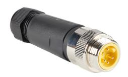
ZIPport connector, field-wireable, 7/8in - 16 UN2 thread barrel 5-pin male axial, accepts cable diameter size 5-13mm, 20 - 14 AWG, North American color code, screw terminal connection, IP67.
