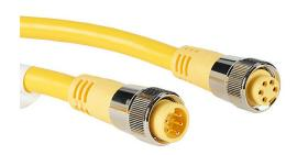
ZIPport connection cable, 7/8in - 16 UN2 thread nut 5-pin male axial to 7/8in - 16 UN2 thread nut 5-pin female axial, PVC outer jacket, yellow, nickel-plated brass connector, 19.6ft/6m cable length, IP67.
