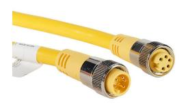
ZIPport connection cable, 7/8in - 16 UN2 thread nut 5-pin male axial to 7/8in - 16 UN2 thread nut 5-pin female axial, PVC outer jacket, yellow, nickel-plated brass connector, 6.5ft/2m cable length, IP67.
