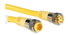
ZIPport connection cable, 7/8in - 16 UN2 thread nut 5-pin male axial to 7/8in - 16 UN2 thread nut 5-pin female axial, PVC outer jacket, yellow, nickel-plated brass connector, 32.8ft/10m cable length, IP67.
