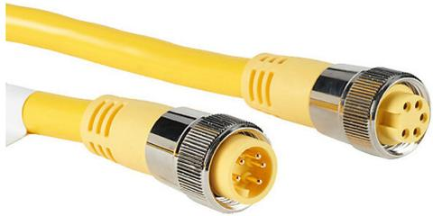
ZIPport connection cable, 7/8in - 16 UN2 thread nut 5-pin male axial to 7/8in - 16 UN2 thread nut 5-pin female axial, PVC outer jacket, yellow, nickel-plated brass connector, 32.8ft/10m cable length, IP67.
