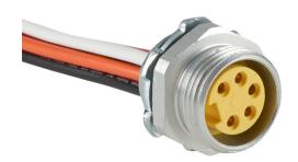
ZIPport bulkhead connector, 7/8in 5-pin female to pigtail, 16 AWG, 0.9ft/0.3m cable length, ether-based polyurethane conductor insulation material, IP67.
