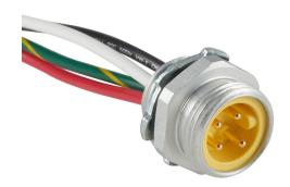
ZIPport bulkhead connector, 7/8in 4-pin male to pigtail, 16 AWG, 0.9ft/0.3m cable length, ether-based polyurethane conductor insulation material, IP67.
