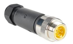
ZIPport connector, field-wireable, 7/8in - 16 UN2 thread barrel 4-pin male axial, accepts cable diameter size 5-13mm, 20 -14 AWG, North American color code, screw terminal connection, IP67.
