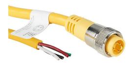
ZIPport connection cable, 7/8in - 16 UN2 thread nut 4-pin male axial to pigtail with North American color code, PVC outer jacket, yellow, nickel-plated brass connector, 13.1ft/4m cable length, IP67.
