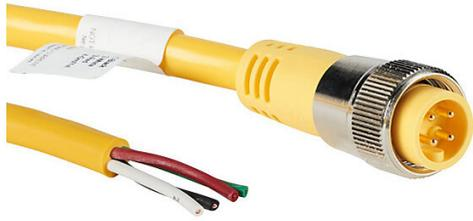
ZIPport connection cable, 7/8in - 16 UN2 thread nut 4-pin male axial to pigtail with North American color code, PVC outer jacket, yellow, nickel-plated brass connector, 6.5ft/2m cable length, IP67.
