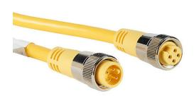
ZIPport connection cable, 7/8in - 16 UN2 thread nut 4-pin male axial to 7/8in - 16 UN2 thread nut 4-pin female axial, PVC outer jacket, yellow, nickel-plated brass connector, 19.6ft/6m cable length, IP67.
