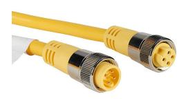
ZIPport connection cable, 7/8in - 16 UN2 thread nut 4-pin male axial to 7/8in - 16 UN2 thread nut 4-pin female axial, PVC outer jacket, yellow, nickel-plated brass connector, 13.1ft/4m cable length, IP67.
