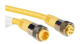
ZIPport connection cable, 7/8in - 16 UN2 thread nut 4-pin male axial to 7/8in - 16 UN2 thread nut 4-pin female axial, PVC outer jacket, yellow, nickel-plated brass connector, 32.8ft/10m cable length, IP67.
