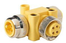
ZIPport T-coupler, (2) 4-pole female 7/8in - 16 UN2 nuts to 4-pole male 7/8in - 16 UN2 barrel, parallel distribution.
