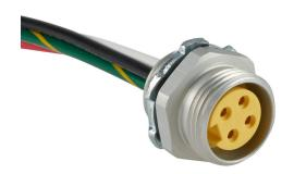
ZIPport bulkhead connector, 7/8in 4-pin female to pigtail, 16 AWG, 0.9ft/0.3m cable length, ether-based polyurethane conductor insulation material, IP67.
