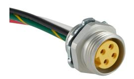
ZIPport bulkhead connector, 7/8in - 16 UN2 thread barrel 4-pin female to pigtail, 16 AWG, 0.9ft/0.3m cable length, PVC conductor insulation material, North American color code. Mounting nut(s) included.
